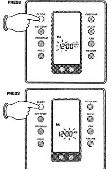
Step 2: Press the CLOCK button again and "12:" (hours) and "AM" or "PM" will flash. Use the DECREASE or INCREASE button to change the flashing symbol to the current hour making sure the hour has the proper AM or PM designation.
